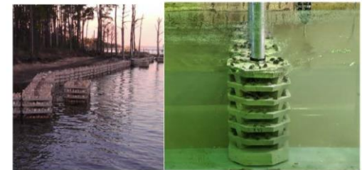
Figure 1. Comparison between installed Living Wave Barrier and 1 to 5.16 scale model.
